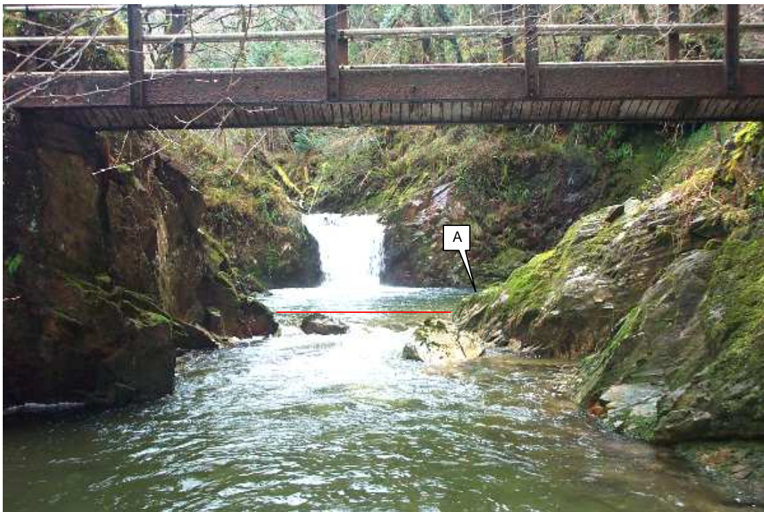
Figure 3.33: Afon Wen hydrograph recording site. The water depth recorder is located in the pool at location A. Flow is measured at the pool outlet along the section shown in red.
