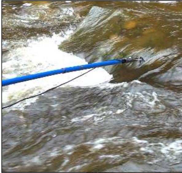
Figure 3.26: (left) Flow meter in position above the river channel. (below) Flow velocity measurement in progress
