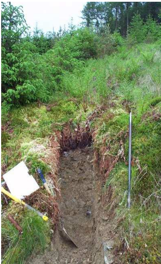
Figure 3.41(a) Site prepared for instrumentation, showing peat soil on glacial till, Pared yr Ychain
