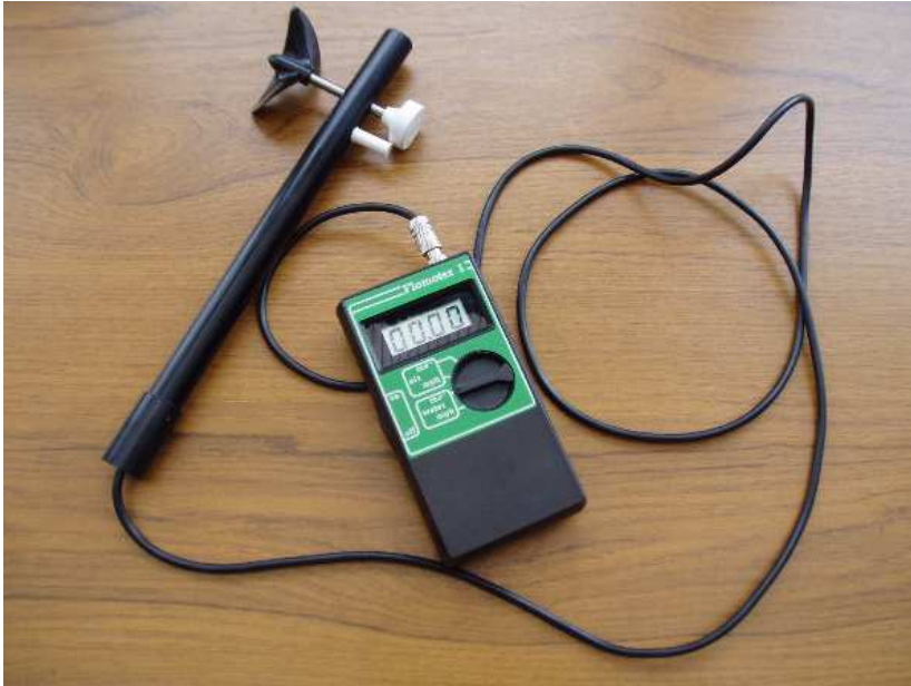
Figure 3.25: Propeller flowmeter used in hydrograph site calibration
