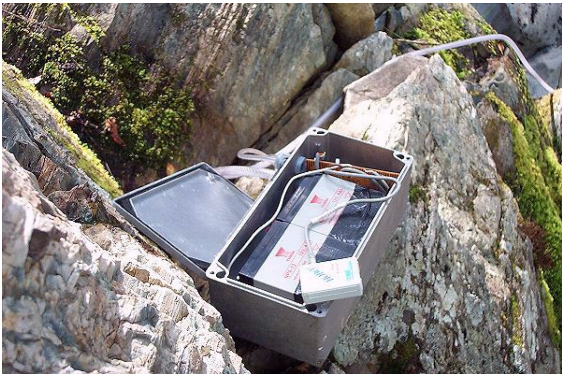
Figure 3.23: Barometric water depth recorder
